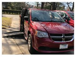
Here is a picture of my van. This is an adaptive van. It has an automated folding ramp. Using my wheelchair, I enter the van. No one needs to lift me into the vehicle or position me in a car seat. I obtained my van via a loan
